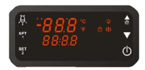
The thermostat is equipped with a **child-lock** device. To activate this function, press the "up"  $\triangle$  and "down"  $\checkmark$  keys simultaneously. After about 3 seconds, the word "Pof" flashes. Do the same operation to unlock the control panel. After approximately 3 seconds, "Pon" flashes.
